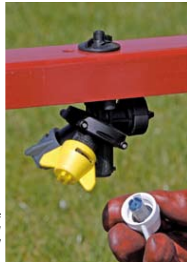
TRIPLET nozzle holders with filters and built in non-drip check valve are standard.
