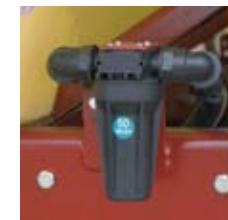
In-line pressure filters for HLC system
